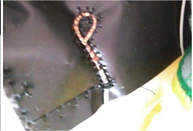
Fig. 8. Electric wire connected to Velostat.
