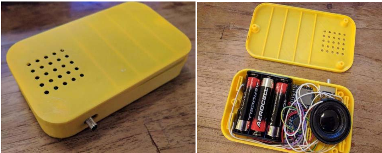
Fig. 14 and 15. Actual print of the casing, with all electronics integrated.
