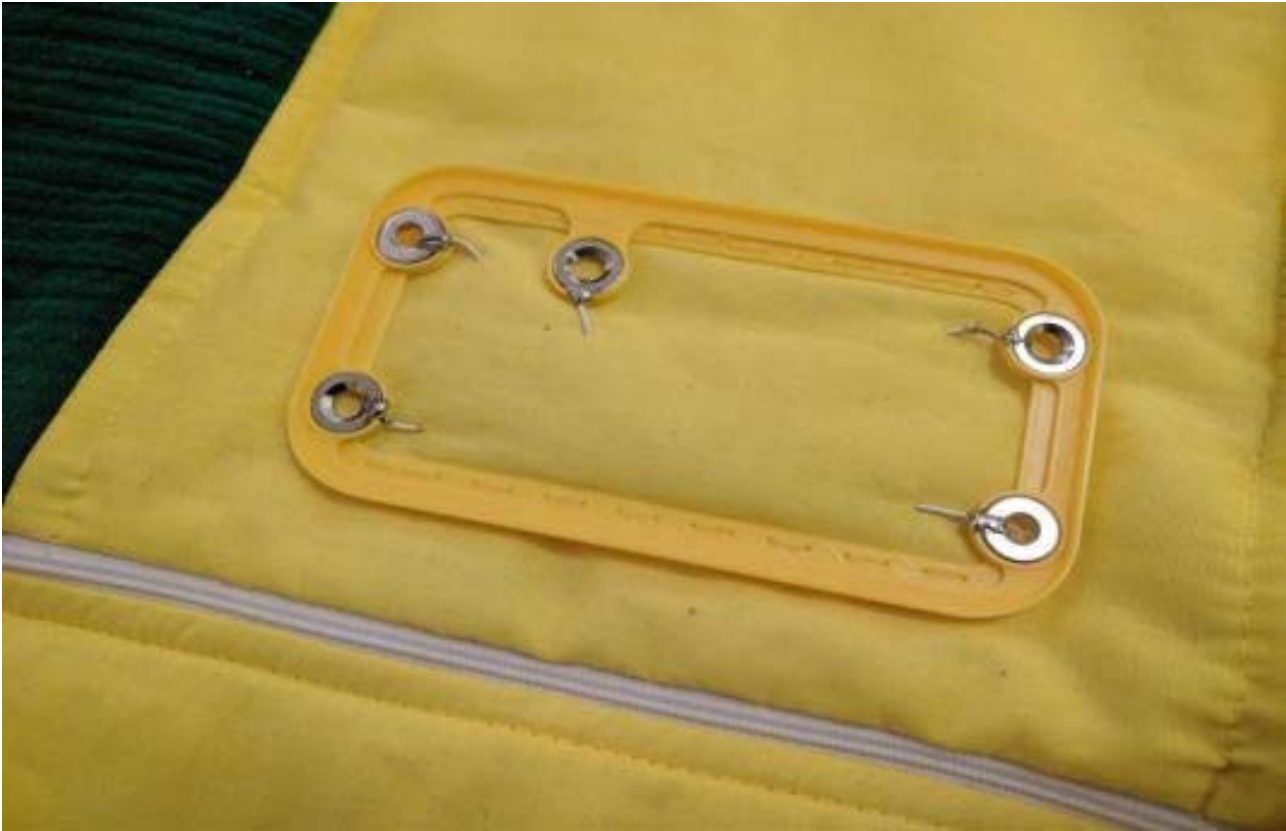
Fig. 16. Five magnetic connection points on the interactive playmat.
